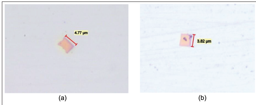
Figure 6. Inclusion Size of Precipitated TiN at the Same Location (W 1/2 -C) in (a) Low Cooling Rate (b) High Cooling Rate.
