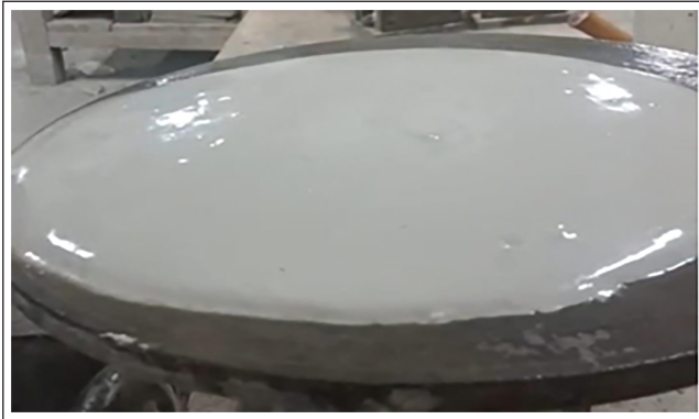
Figure 4. Flow Table Test of Cupola Slag-Based Cement.
